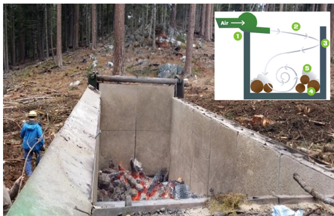
Fig. 6. Air-Curtain Burner (1. Air manifold; 2. Air curtain; 3. Firebox refractory wall; 4. Wood waste or fuel; 5. Smoke and particulates. Image from www.airburners.com ).
