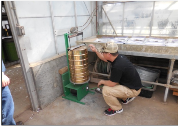
Figure 2. Size distribution of screened materials from each size class: under, accept and over using an oscillating sieve shaker.
