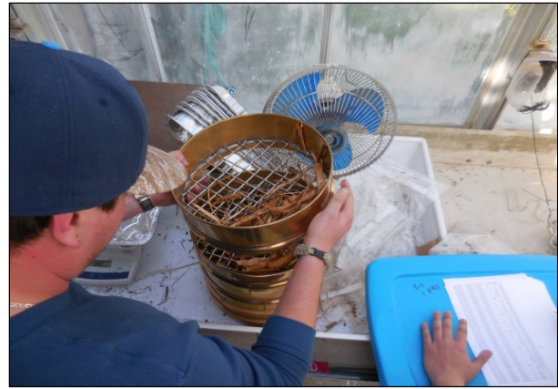
Figure 2. Size distribution of screened materials from each size class: under, accept and over using an oscillating sieve shaker.
