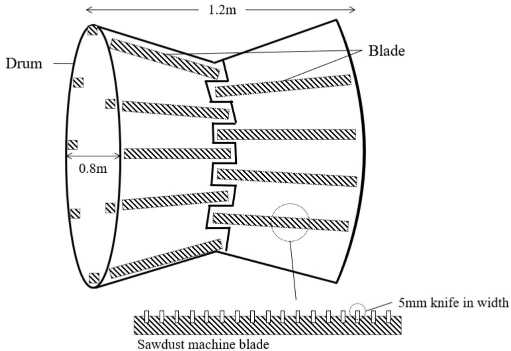
Figure 1. The principle of a sawdust machine drum and knives. The drum carries 18 -19 rows of 37 blades. Rows are equally spaced on the drum surface. The blades is equipped 16-17 knives of 5mm. The sawdust machine version carries 582 knives in the drum.
