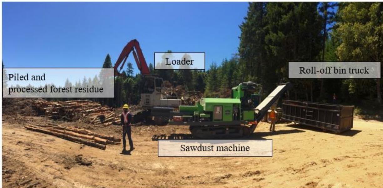
Figure 2. Overview of the sawdust machine testing. The loader fed the left side of the sawdust machine and sawdust was conveyed up the ramp on the right side of the machine into a bin. The sawdust machine required an operator, to monitor the drum's revolutions per minute and control the in-feed conveyor.
